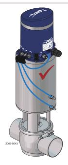
(2) Verify that the air exhaust plug points downwards as indicated by the arrow to avoid water ingress in the pneumatic system. You can rotate the exhaust plug until it points in the right direction.
